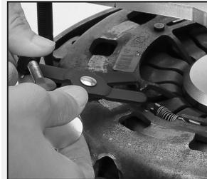
If the old clutch cover is to be reused, it must first be reset. The adjuster ring can be turned back with clutch resetting tool together with clamping tool.
