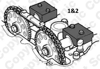
Lock the balancer shaft chain tensioner in its retracted position using
