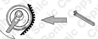
Component 2 - Camshaft Alignment Strap (SOHC) Component 2 is used to lock the camshaft in its timed position. Fits from the gear box end of the camshaft with cam cover removed.
