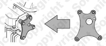
Component 5 - Crankshaft Alignment Tool Use component 5 to lock the crankshaft in its timed position once the crankshaft pulley has been removed.
