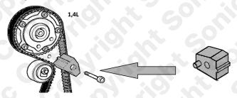
Component 5 - Crankshaft Alignment Tool
