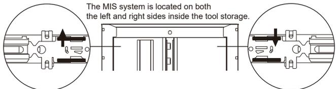
After removing the first drawer, push the MIS switch on the right side downward and the MIS switch on the left side upward. Then, you can remove the other drawers.
