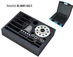
Suitable for wheel bearing units without centre bore for example on rear axles with wheel bearing dia. 85 mm with Toyota ProAce; Peugeot Expert, Traveller; Citroen Jumpy, Spacetourer, and many more. Also suitable for conventional wheel bearing units and hole circle Ø 5x108, 5x112 mm.
