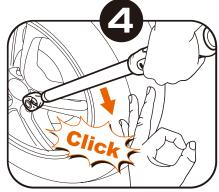
Hold the handle firmly in the middle to move the torque wrench clockwise carefully and stop immediately after "click".
