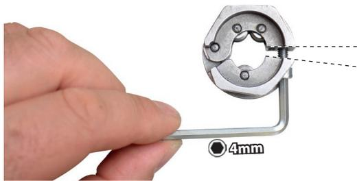
📷 2: Place the re-threading tool correctly on the thread.
