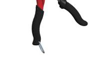
**3.** Put the nut into the riveting hole, close the handle to deform the nut to rivet in place.
